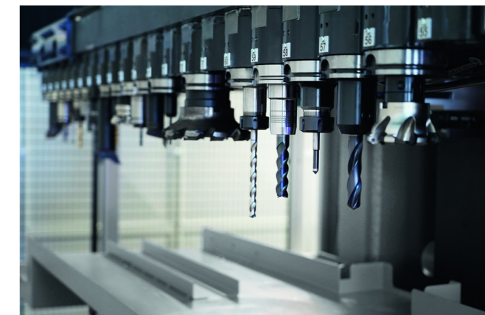
Tool magazine at the rear in a right angle to the column
