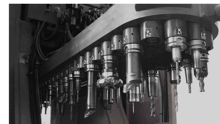
Tool magazine integrated in the machine column
